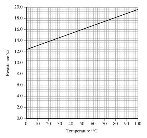
(i) The graph shows that resistance is **not** directly proportional to temperature in °C. State how the graph shows this.
