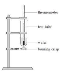
Once the crisp had finished burning, the student recorded the final temperature of the water. The experiment was carried out three times using a crisp of the same mass.
