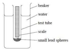
The test tube is displaced downwards and released. After release the test tube moves with simple harmonic motion.
