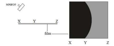
A second film is covered by strips of card and aluminium as shown.
