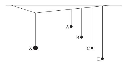
After a short time C is observed to have the largest amplitude of oscillation.
