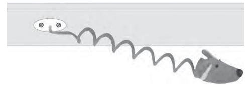
(a) Show that the acceleration of the mouse, a, is given by  $a = -\left(\frac{k}{m}\right)x$ , where k is the stiffness of the spring.
