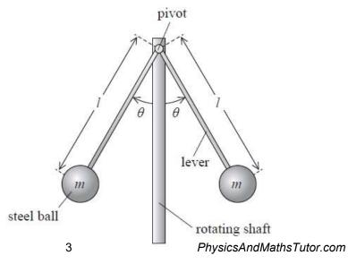
Two steel balls, each of mass m, can move apart at the end of levers that are freely pivoted. As the vertical shaft rotates, the two steel balls move apart so that the angle between the lever and the vertical is  $\theta$ .
