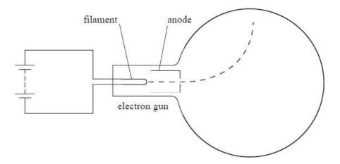
Electrons are released by a filament and accelerated towards the anode, producing a beam. A magnetic field is applied, deflecting the beam as shown.
