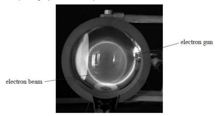
The fine beam tube contains helium gas at very low pressure. When electrons strike the helium atoms the resulting excitation is responsible for the glow tracing the path of the electron beam.
