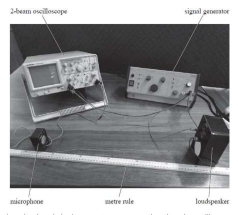
When the loudspeaker is switched on, two traces are produced on the oscilloscope, one directly from the signal generator and the other from the microphone.
