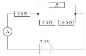
The ammeter displays a current of 0.50 A.
