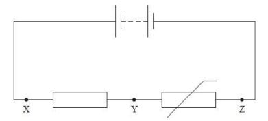
A potential divider circuit can be created by making connections to a secondary circuit across the resistor (XY) or across the thermistor (YZ). As the temperature changes, the potential differences (p.d.) across XY and YZ both change.
