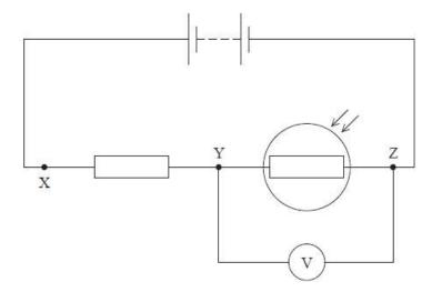
The fixed resistor has a resistance of 1.20 k $\Omega$ . The battery has an e.m.f. of 12.0 V and negligible internal resistance. Initially the circuit is set up in a darkened room, and the voltmeter displays a reading of 4.71 V. When a light is shone directly onto the LDR, the voltmeter reads 2.16 V. Calculate the change in resistance of the LDR when the light is shone onto it.
