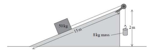
Determine whether the maximum efficiency of the machine was greater than 90%.
