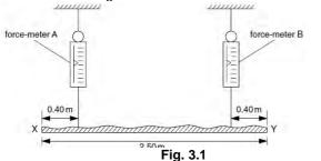
When the plank is horizontal, force-meter A records 570 N.
