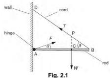
The rod has weight W and the centre of gravity of the rod is at C. The rod is held in equilibrium by a force T in the cord and a force F produced at the hinge. (a) Explain what is meant by (i) the *centre of gravity* of a body, [2] (ii) the *equilibrium* of a body. [2] (b) The line of action of the weight *W* of the rod passes through the cord at point P.
