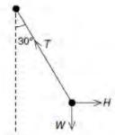
The tension in the string of the pendulum is T. The weight of the pendulum bob is W.
