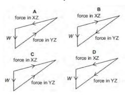
35. A uniform ladder rests against a vertical wall where there is negligible friction. The bottom of the ladder rests on rough ground where there is friction. The top of the ladder is at a height h above the ground and the foot of the ladder is at a distance 2a from the wall
