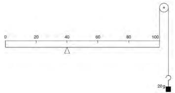
At which mark on the rule must a 50 g mass be suspended so that the rule balances?
