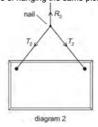
In both cases, a string is attached to the same points on the picture and looped symmetrically over a nail in a wall. The forces shown are those that act on the nail.
