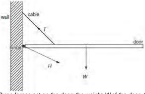
Three forces act on the door: the weight W of the door, the tension T in the cable, and the force  $\hat{H}$  at the hinge. Which list gives the three forces in increasing order of magnitude?
