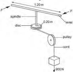
What is the minimum force F, applied to each end of the lever, that could lift the weight?
