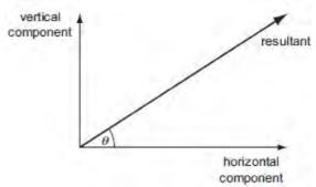
The horizontal component is 20.0 N and  $\theta$  = 30°. What is the vertical component?
