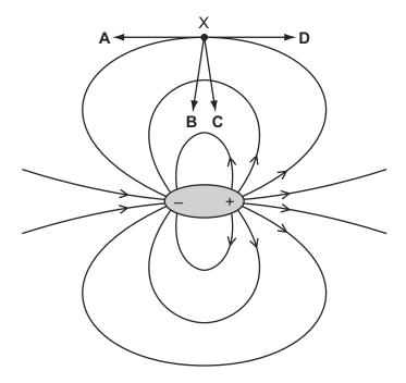
32 Lightning can occur between a charged cloud and the Earth's surface when the electric field strength in the intervening atmosphere reaches 25 kN C<sup>-1</sup>. The diagram shows the electric field between the base of a cloud and the Earth's surface.
