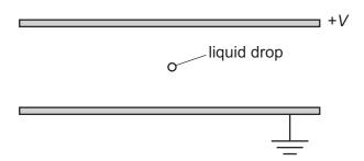
A small charged liquid drop, midway between the plates, is held in equilibrium by the combination of its weight and the electric force acting on it.
