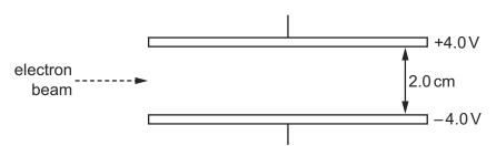
The upper plate has an electrical potential of  $+4.0\,\mathrm{V}$ , and the lower plate has an electrical potential of  $-4.0\,\mathrm{V}$ .
