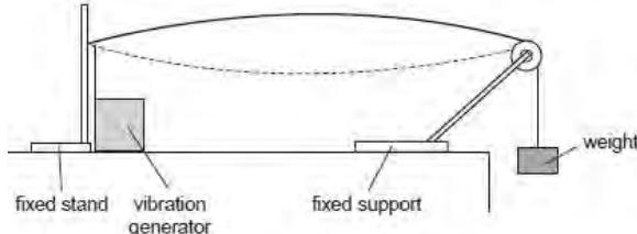
A vibration generator is attached to the wire near the clamped end. A stationary wave with one loop is produced. The frequency of the vibration generator is  $f$ .
