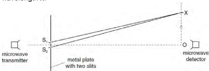
The detector is moved from O in the direction of the arrow. The signal detected decreases until the detector reaches the point X, and then starts to increase again as the detector moves beyond X.
