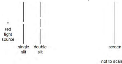
Fringes are formed on the screen. The distance between successive bright fringes is found to be 4 mm. Two changes are then made to the experimental arrangement. The double slit is replaced by another double slit which has half the spacing. The screen is moved so that its distance from the double slit is twice as great.
