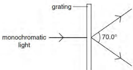
The spacing of the slits in the grating is  $1.00 \times 10^{-6}$  m. The angle between the first order diffraction maxima is  $70.0^\circ$ .
