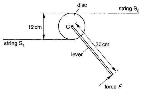
The disc is free to rotate about an axis normal to its plane. The axis passes through the centre C of the disc.
