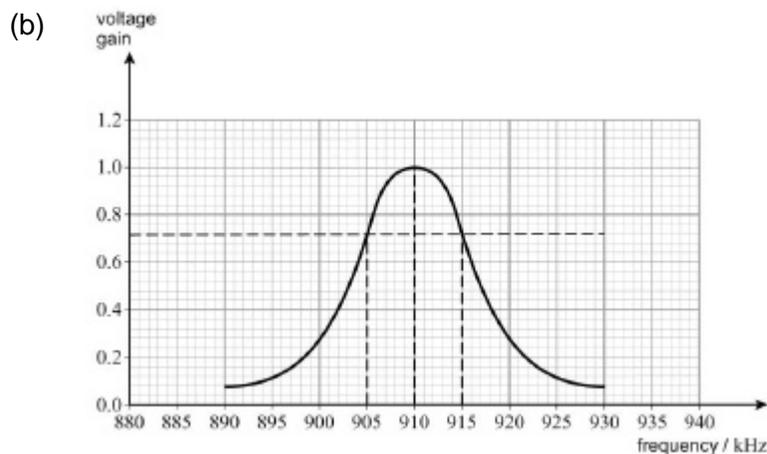
*General shape around  $f_0$  and to max of 1.0 on relative voltage gain axis*
