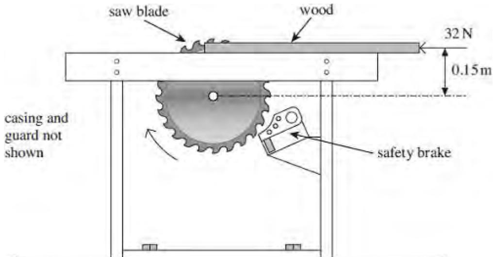
A horizontal force of  $32 \text{ N}$  is needed to push a piece of wood into the saw. The force acts on the blade at an effective radius of  $0.15 \text{ m}$ .
