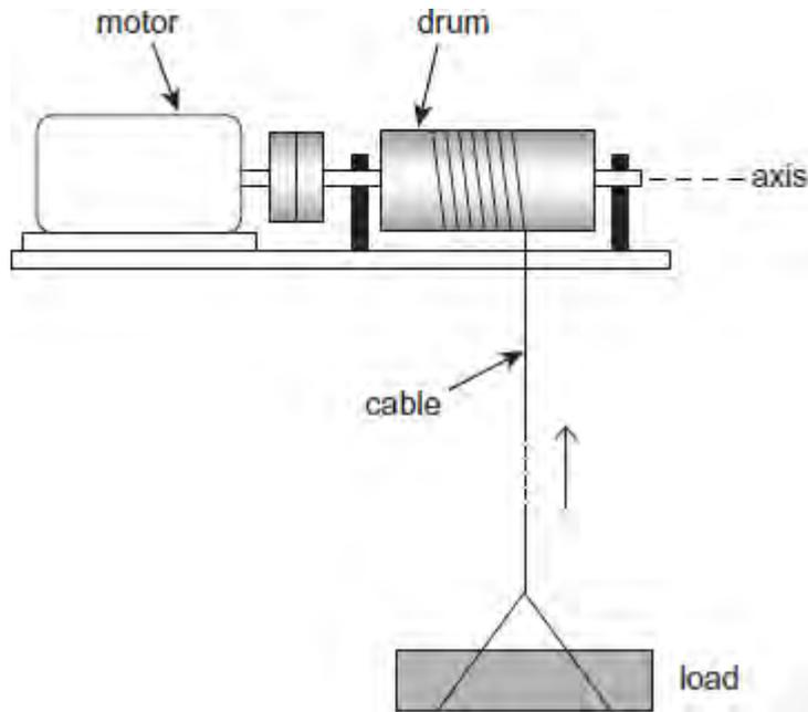
The drum, axle and other rotating parts have a moment of inertia about the axis of rotation of  $7.4 \text{ kg m}^2$ , and the mass of the load is  $85 \text{ kg}$ . The drum has a radius of  $0.088 \text{ m}$ .
