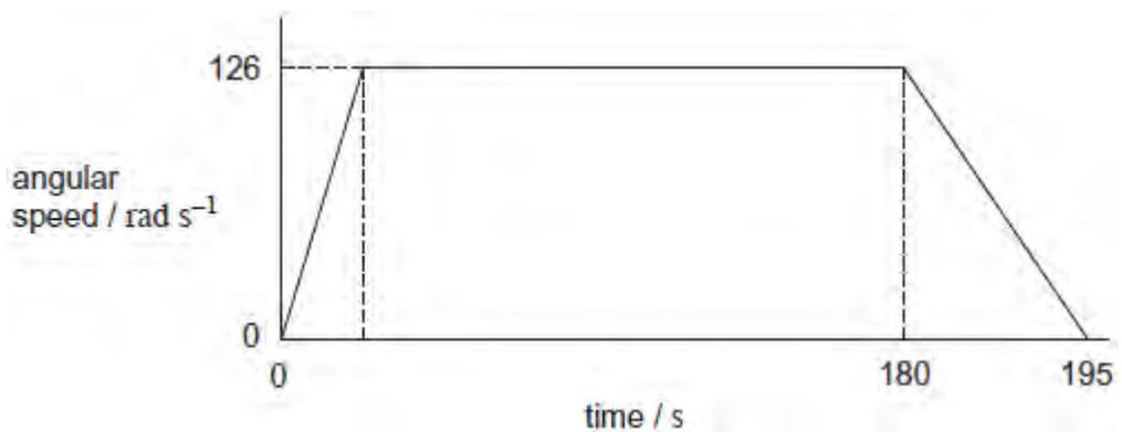
The motor provides a torque of  $8.80 \text{ N m}$  to accelerate the drum to  $126 \text{ rad s}^{-1}$ . The drum rotates at  $126 \text{ rad s}^{-1}$  until near the end of the spin cycle, when the drum decelerates uniformly to zero angular speed in 15 seconds. Friction at the bearings
