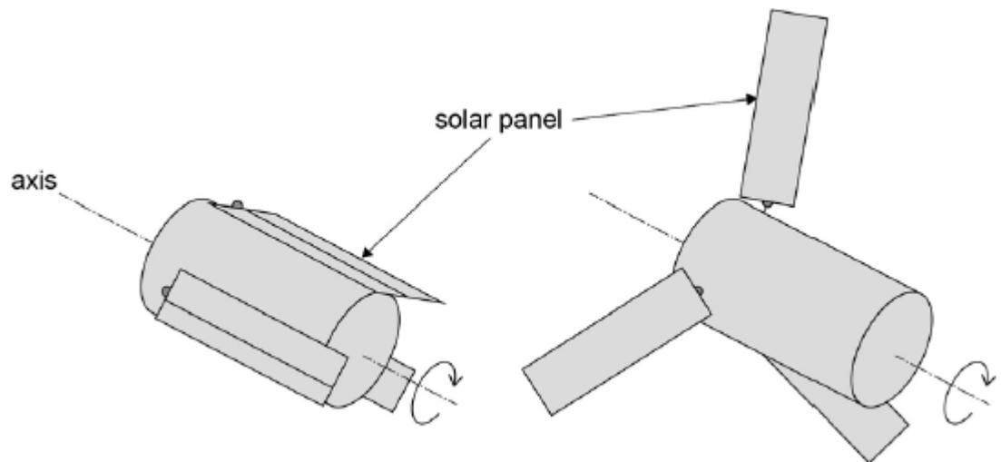
Just before it is released into space, the satellite is spun to rotate at  $5.2 \text{ rad s}^{-1}$ . Once released, the solar panels are extended as shown in **Figure 2**.
