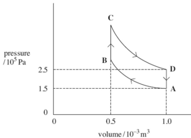
(a) (i) Show that the temperature of the air at point D is 500 K.
