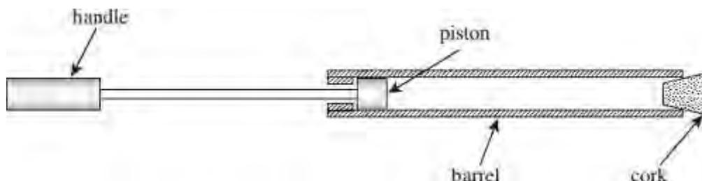
The figure above shows the gun before it is 'fired'. The air in the barrel is at a pressure of  $1.0 \times 10^5$  Pa, a temperature of 290 K and the volume is  $2.1 \times 10^{-5}$  m<sup>3</sup>.
