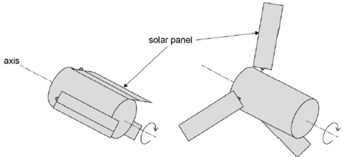
Just before it is released into space, the satellite is spun to rotate at  $5.2 \text{ rad s}^{-1}$ . Once released, the solar panels are extended as shown in **Figure 2**.
