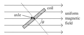
A coil of 50 turns has a cross-sectional area of  $4.2 \times 10^{-3}$  m<sup>2</sup>. It is placed at an angle to a uniform magnetic field of flux density  $2.8 \times 10^{-2}$  T, as shown in the diagram, so that angle  $\vartheta = 50^{\circ}$ .
