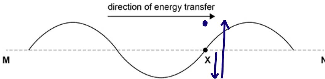
The wave has a frequency of 5.0 Hz, a wavelength of 1.0 m and an amplitude of 0.20 m.
