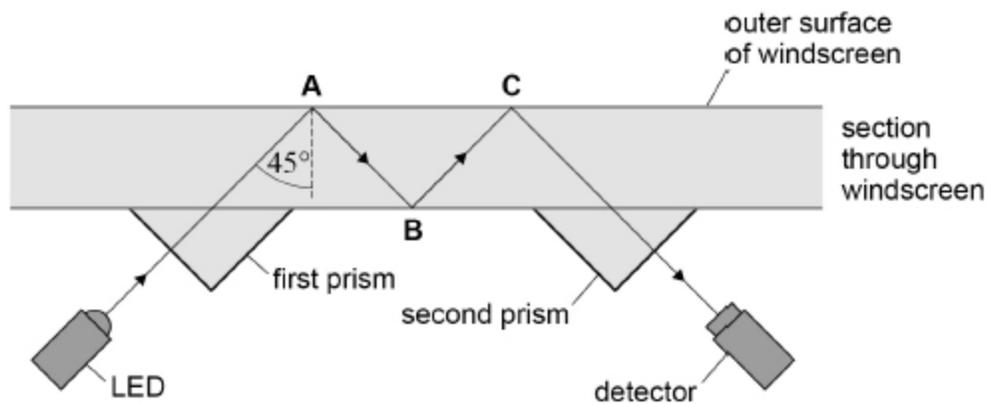
A light ray travels from the light-emitting diode (LED) through the first prism and into the windscreen. The ray reflects off the surfaces of the windscreen at **A**, **B** and **C** and then passes through the second prism into the detector.
