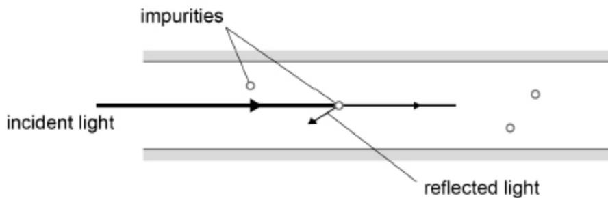
Earthquakes bend the optical fibre slightly, as shown in **Figure 4**. This changes the amount of reflected light.
