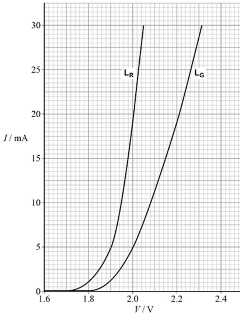
When the linear part of the characteristic is extrapolated, the point at which it meets the horizontal axis gives the activation voltage  $V_A$  for the LED.
