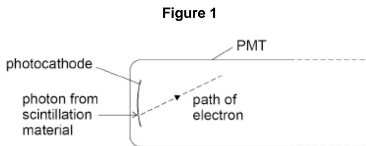
The longest wavelength of light that releases an electron from this photocathode is 630 nm.
