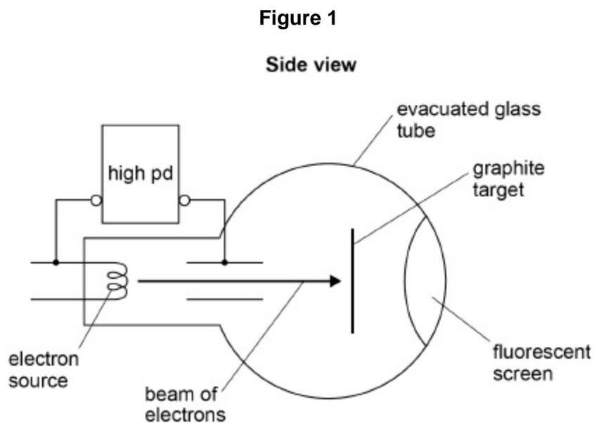
An electron beam is incident on a thin graphite target that behaves like the slits in a diffraction grating experiment. After passing through the graphite target the electrons strike a fluorescent screen.
