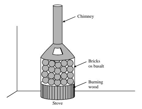
Before use the basalt is tested for resistance to cracking by first heating the bricks to 750°C and then dropping them into cold water.
