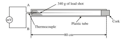
The thermocouple generates only a fraction of a millivolt in experiments of this kind. In order to check this voltage a potential divider is used.
