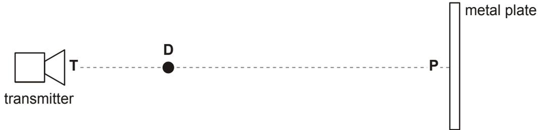
Microwaves leave the transmitter and move in a direction **TP** which is at right angles to the metal plate. A standing (stationary) wave is formed between **T** and **P**.
