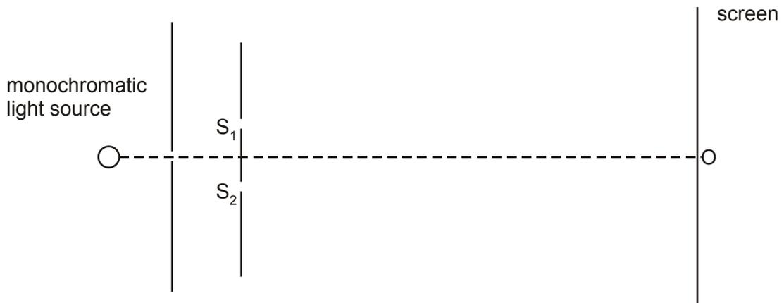
In a darkened room, a double slit ( $S_1S_2$ ) is placed in front of a narrow single slit situated in front of a monochromatic (one frequency only) light source.
