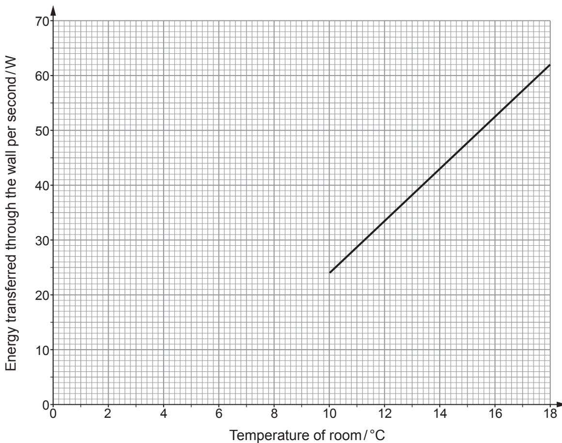
Use the graph to determine the temperature outside the building and the  $U$  value of the wall. [3]
