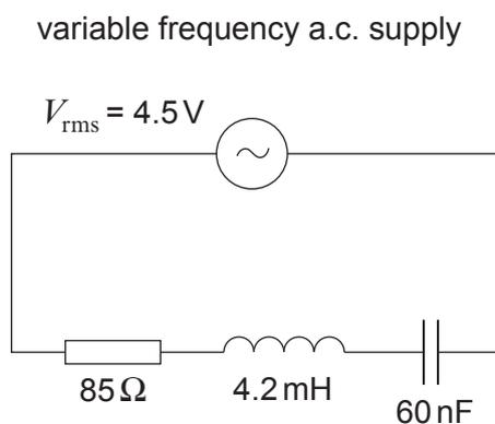
(i) Show that the resonance frequency of the circuit above is approximately 10 000 Hz. [1]
