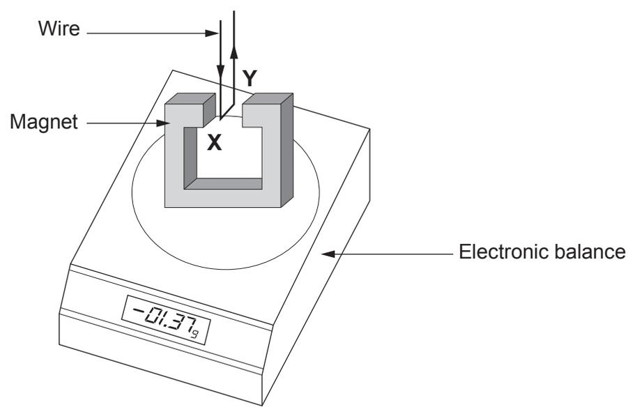
The portion **XY** of the wire which is in the magnetic field, has been placed carefully so that the current is from **X** to **Y** at  $90^\circ$  to the direction of the magnetic field. While there is no current, the balance is reset to display 00.00g. When there is a current in the direction shown, the electromagnetic force results in a negative reading on the display of the balance. This signifies an upward force on the magnet and a downward force on the wire.
