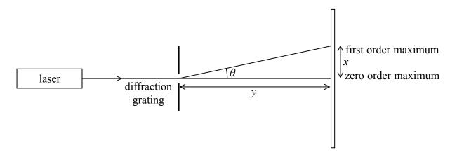
The student measures x, the distance between the zero order maximum and the first order maximum, and y, the distance between the slit and the screen.
