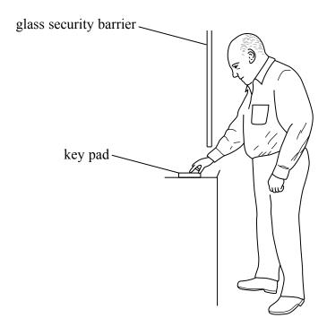
When standing as shown in the diagram, refraction of light through the glass means that the motorist is unable to see the key pad without moving his head to see under the glass.
