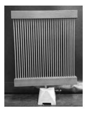
The filter is placed between a microwave source and a detector, which detects a strong signal.
