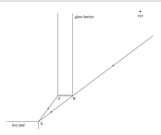
(a) The diagram shows rays from the key pad. The light travelling initially along the path XA, which then passes through the glass, does not reach the motorist's eye. Assume no light passes through the surface AB.
