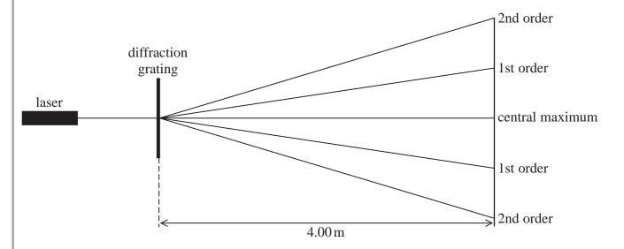
The student measured the distance between the central and a 2nd order maximum as 1350 mm. The diffraction grating had 300 slits mm<sup>-1</sup>.
