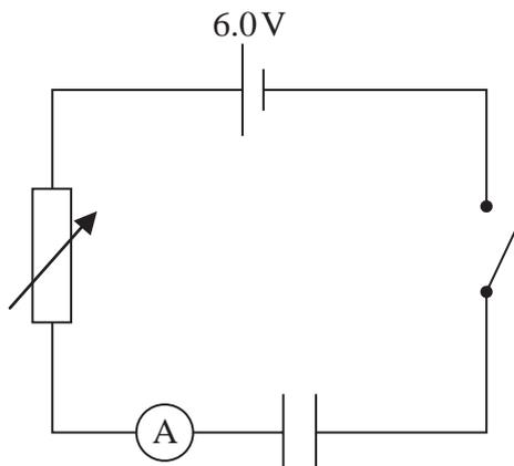
(a) When the switch is closed there is a maximum current, which decreases to zero over a period of time as the capacitor charges. Explain why.
