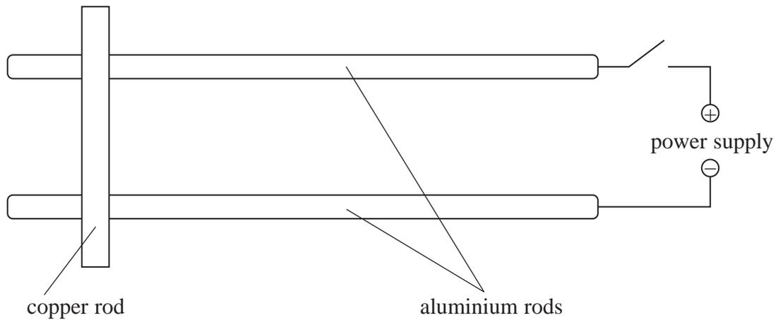
The apparatus is placed in a magnetic field. When the switch is closed, the copper rod rolls along the aluminium rods.
