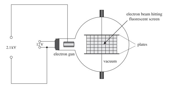
(a) The electron gun consists of a hot metal filament and a positively charged anode. Explain how this produces a beam of electrons.
