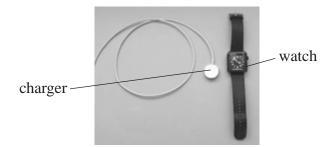
Induction charging does not require a metal connection between the charger and the device. The battery in the watch is charged by placing the watch on top of the charger.
