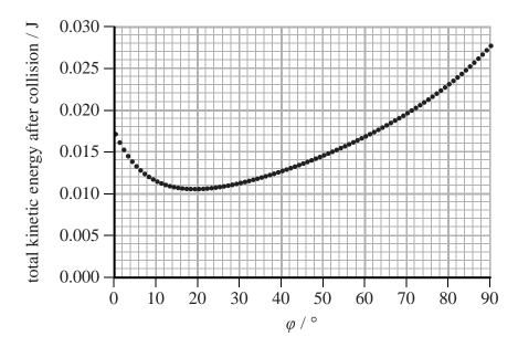
Measure  $\varphi$  from the photograph and use the graph to suggest why the angle between the paths is not  $90^{\circ}$ .
