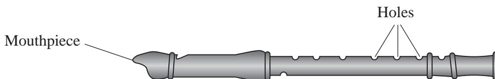
The length  $l$  of the vibrating air column is changed by covering the holes. This changes the frequency  $f$  of the sound produced.
