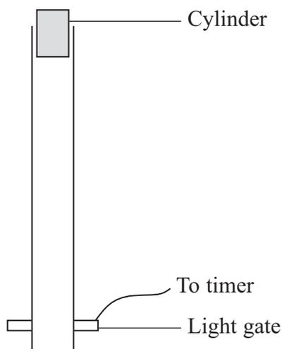
The light gate measures the time taken for the cylinder to pass through it. This time  $t$  is used to calculate the velocity of the cylinder at a distance  $s$  from the top of the tube.
