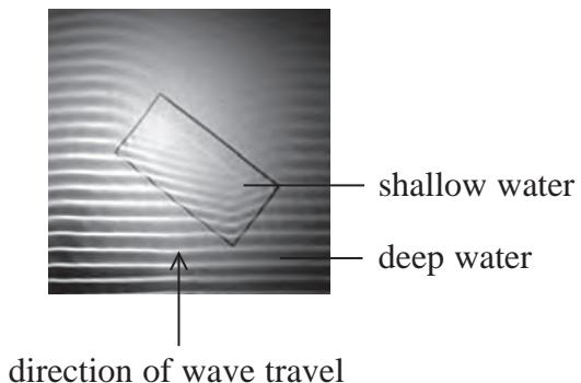
It is observed that the waves are closer together as they move through the shallow water. This is because the waves in the shallow water
