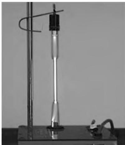
A high potential difference is applied across the tube and a spectrometer can be used to produce a visible line spectrum, as shown below.
