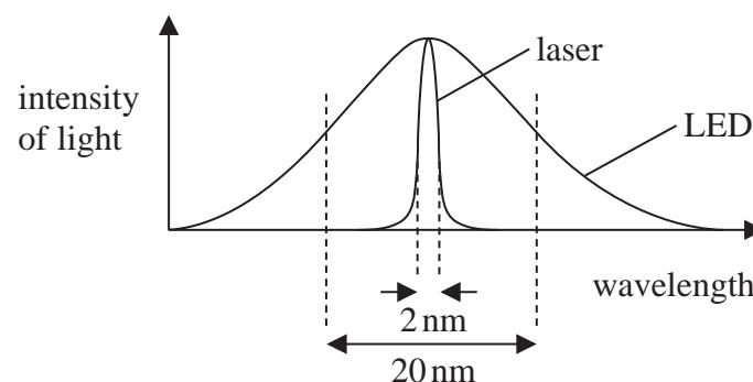
Light of different wavelengths will travel at different speeds along the fibre.
