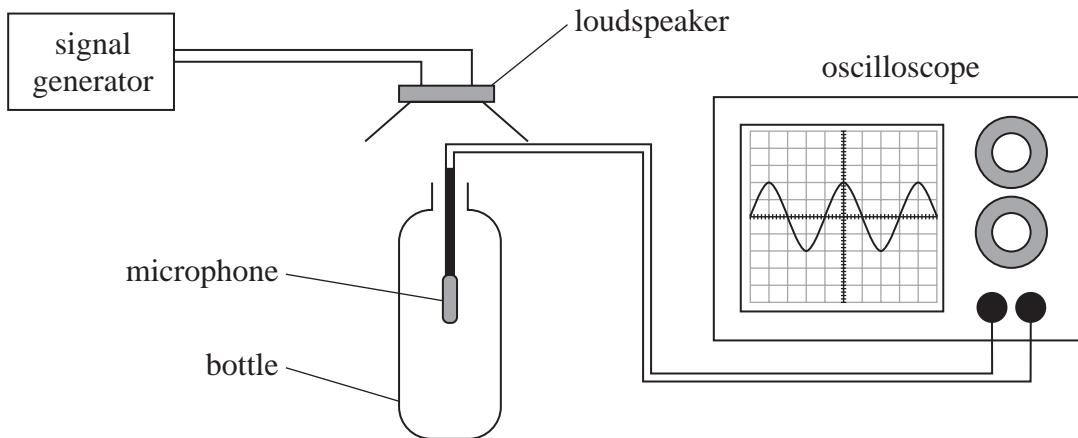
The signal generator was adjusted until a loud sound was heard at a particular frequency, known as the resonant frequency.
