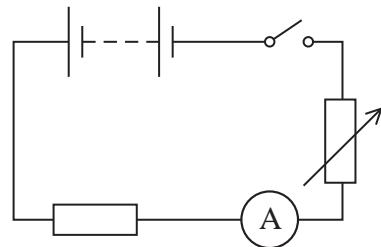
A student investigated whether the temperature rise of the water  $\Delta\theta$  was proportional to the current  $I$  in the resistor. For each value of current, the student refilled the beaker with water at the same initial temperature.
