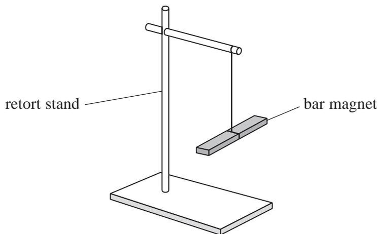
The magnet lined up with the magnetic field of the Earth.
