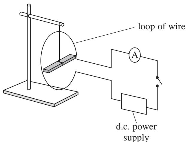
When the switch was closed, there was a current  $I$  in the loop of wire and the time period  $T$  of the oscillations decreased.
