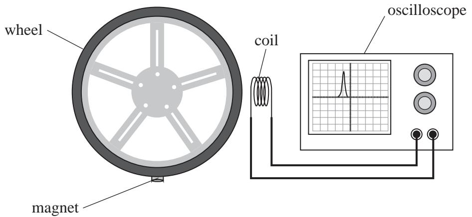
A magnet is attached to the edge of the wheel. When the magnet passes the coil, a single pulse is displayed on the oscilloscope screen.
