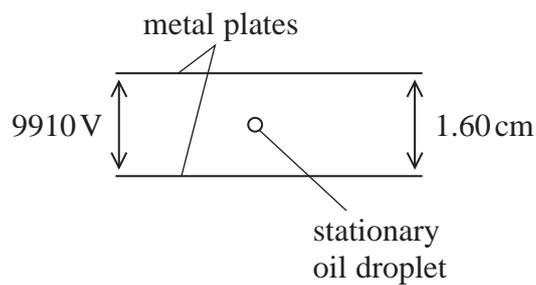
Calculate the charge on the oil droplet.
