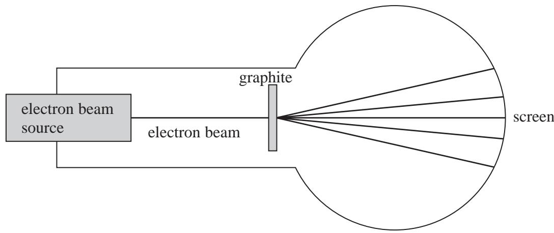
The diffraction pattern seen on the curved screen is shown below.
