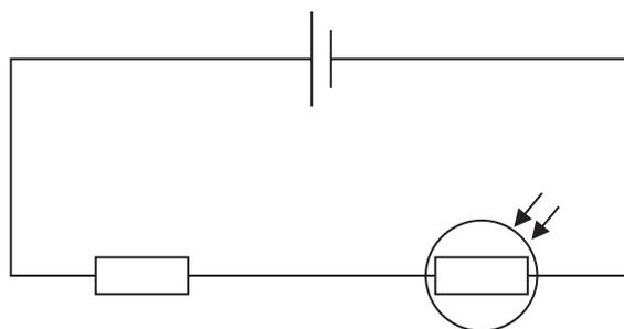
The intensity of the light incident on the LDR is increased.
