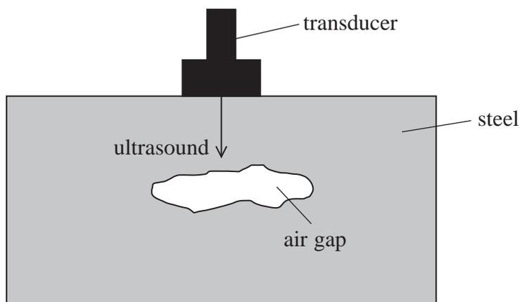
(a) Explain how this arrangement can be used to show whether the RSJ contains an air gap.
