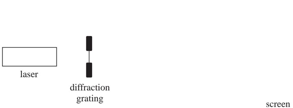
When the laser is switched on, a series of bright dots is seen on the screen.
