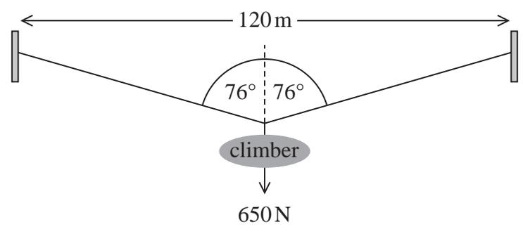
(i) Determine the strain in the rope while it is supporting the weight of the climber.
