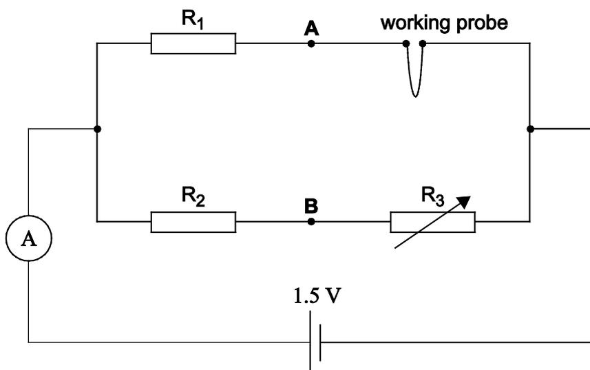
When  $R_3$  is adjusted to a particular value the current in the cell is 0.66 A.
