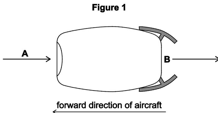
Air enters the engine at **A** and is heated before leaving **B** at a much higher speed.
