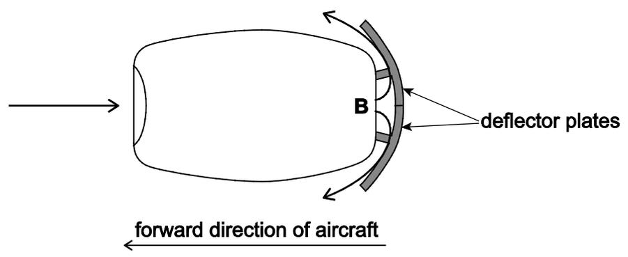
The speed of the air leaving **B** is the same as the speed of the deflected air.
