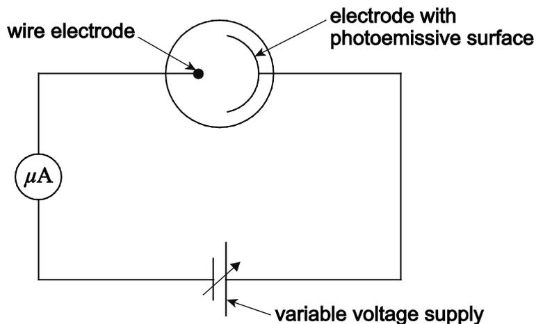
The photoemissive surface has a work function of  $2.1 \text{ eV}$ . The frequency of the electromagnetic radiation the student uses is  $7.23 \times 10^{14} \text{ Hz}$ .
