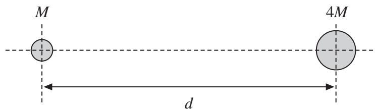
The resultant gravitational field strength is zero along the line between their centres at a distance  $y$  from the centre of the star of mass  $M$ .
