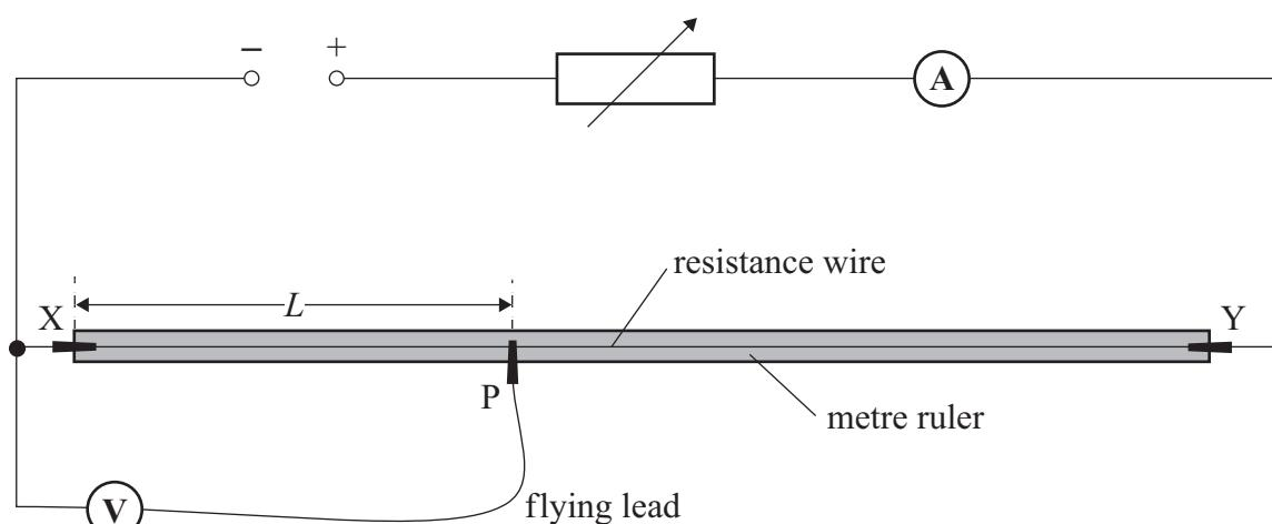
If a resistance wire of a different gauge and/or a different metal is used, the voltage of the power supply should be set to a value approximately numerically equal to the resistance of the wire in ohms to give a current of about 1 A with the variable resistor set at zero resistance. Centres using continuously varying power supplies should inform candidates that the variable resistor will not be required.
