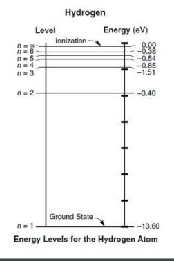
The coloured lines we see above arise from electrons falling between some of these states shown to the left. All transitions will emit a photon of some type of electromagnetic radiation, however, only four of the emissions are visible.
