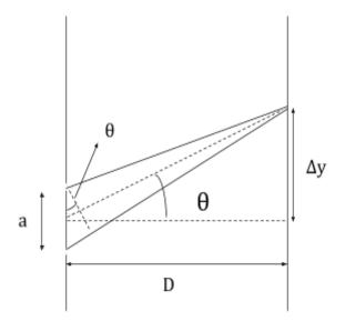
This is a diagram of the double slit experiment. When the two rays meet on the screen, they either undergo constructive or destructive interference or some other partial interference.
