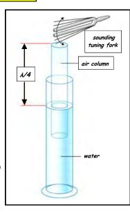
By further increasing the length of the air column, a **second** resonance position is obtained.
