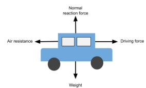
A free-body diagram will show you how each of the forces acting on the object compare with each other. In this example, all the arrows look equal therefore we know that the car is travelling at a constant velocity.
