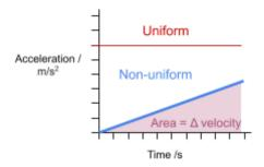
**Acceleration-time graphs** represent the change in acceleration over time. The area under the graph is change in velocity.
