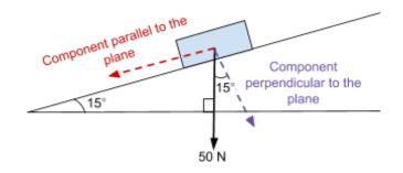
Using the fact that the angles in a triangle add up to 180°, you can see that the angle between the component of weight perpendicular to the plane and weight is also 15°. Using this fact and the useful hint in red above, you can easily find the components of weight.
