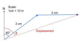
The opposite of adding two vectors is called **resolving vectors**, and is done using trigonometry. It is extremely helpful to do this in certain situations because vectors which are perpendicular don't affect each other, so can be evaluated separately.
