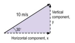
For example, a ball has been fired at a velocity of 10 m/s, at an angle of 30° from the horizontal, find the vertical and horizontal components of velocity.
