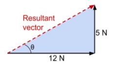
Scale drawing - This should be used when vectors are at angles other than 90°.
