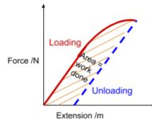
Once a material is stretched beyond its elastic limit, a force-extension graph showing loading and unloading, will not return to the origin, however the loading and unloading lines will be parallel because the material's stiffness is constant, as shown on the left. The area between the loading and unloading line is the work done to permanently deform the material.
