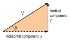
There are formulas to show how to resolve the vector V, into its components x and y.  $x = V \cos \theta$   $y = V \sin \theta$
