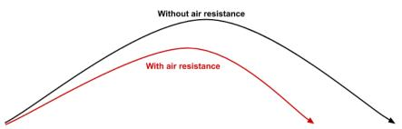
As you can see, with air resistance the maximum height is reached earlier, and the vertical and horizontal distance travelled decreases.
